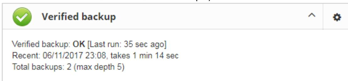
“Database: Verified Backup” checks the free space at the drive with backup destination, and if it detects that there is not enough free disk space, CRITICAL alert will be sent, and current backup will be canceled (if necessary).
