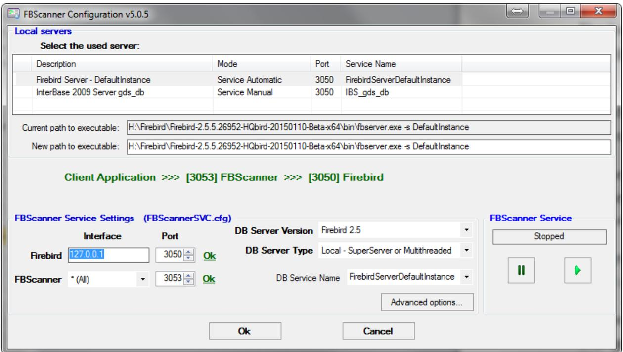
By default Firebird uses port 3050 for network connections. FBScanner works as a transparent TCP proxy – it redirects all SQL traffic from and to Firebird clients to another.
