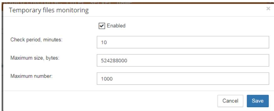
Using configuration dialog you can enable/disable this job, set period and thresholds to the maximum size of temporary files (size of all files) and quantity.
